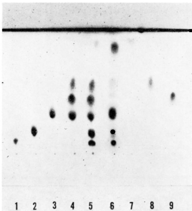
FIG. 2. Thin-layer chromatogram of different reference phospholipids and phospholipids extracted from rat liver. “Basic plate” prepared from silica gel without calcium sulfate. Developing solvent: chloroform–methanol–glacial acetic acid–water 50:25:7:3 (v/v). Detection method: 40% sulfuric acid spray. Compounds: (1) lysolecithin, 10 \mu\text{g} ; (2) sphingomyelin, 15 \mu\text{g} ; (3) lecithin, 15 \mu\text{g} ; (4) mixture of (3), (8), and (9); (5) mixture of (1) to (3) and (7) to (9); (6) phospholipids extracted from rat liver, 120 \mu\text{g} ; spots identified as (from bottom to the top): lysolecithin, sphingomyelin, lecithin, phosphatidyl inositol, phosphatidyl serine, phosphatidyl ethanolamine, and polyglycerophosphatides fused with solvent front band; (7) phosphatidyl ethanolamine (synthetic), 5 \mu\text{g} ; (8) phosphatidyl serine 12 \mu\text{g} ; (9) phosphatidyl inositol, 10 \mu\text{g} .
